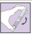
5 Shake the capped tube for 5 seconds. Discard or recycle the funnel.
